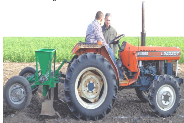
Fig. 2. The used tractor equipped with the manufactured planter.
